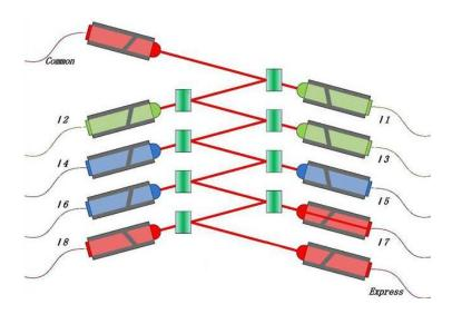
The CCWDM can be used for datacom / telecom network applications using low-cost uncooled lasers. It is available in 4/8/10/12/16/18 channels with an extended port channels.
